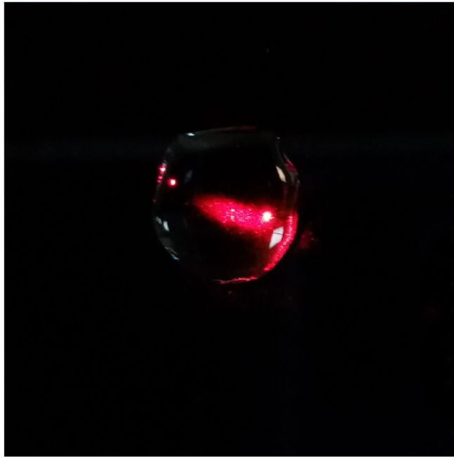
Figure 4.1: Water sample on the Si ATR prism surface. The bright red light is the marker laser spot.
